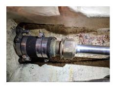
Boats with inboard engines where the drive shaft goes through the hull to turn the prop need some method to prevent water from entering the boat through the drive shaft opening. For over a hundred years a simple method called a stuffing box has been used and is still found on most inboard engine boats. Some boats have a dripless shaft which uses a complex mechanical device to keep water out.
