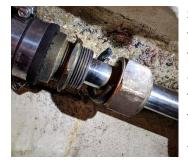
Since the drive shaft on my boat is 1" diameter, I used a spare piece of SS 1" tubing to wrap the packing and measure the lengths for cutting. This is easier than trying to do the measurements and cutting on the actual shaft. The best way to cut the packing is a mitre cut at 45 degrees with a razor knife. This allows the packing to compress tighter and allow less water to flow into the boat. The cuts are made to leave a tight fit around the shaft.
