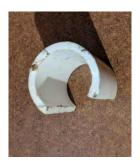
I used a short piece of 1-inch (ID) plastic pipe which was cut to make a snap-on sleeve as a packing tool. Once the packing is just inside the nut, snap the plastic tool onto the shaft and slide it gently into the nut pushing the packing with it, again, without twisting the nut.
