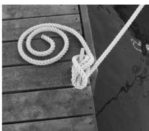
Above: a proper splice fitted well to the cleat.
