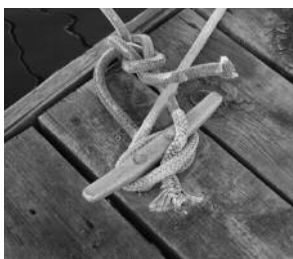
The knot on the left will jam, which is the last thing you want in an emergency.
