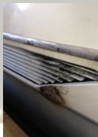
Hot plug melted fiberglass
